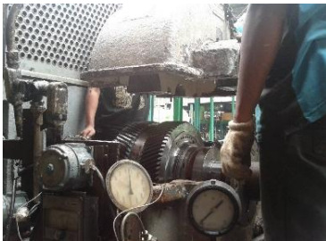
Gambar 5. Saat cover gearbox diangkat
