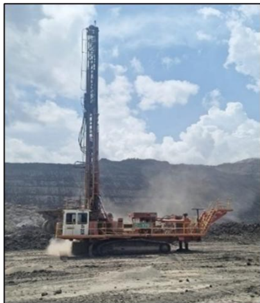
Figure 3. Sandvik D55SP drilling rig
