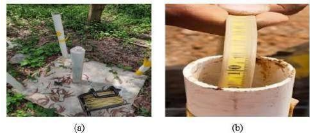
Figure 2. Monitoring Wells in the XYZ Disposal Area (a). Monitoring well photograph, (b). Water level meter photograph
