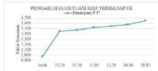
Figure 21. Graph of Groundwater Table Influence on Slope Stability for Cross-Section F-F'
