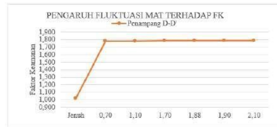
Figure 22. Graph of Groundwater Table Influence on slope Stability for Cross-Section D-D'
